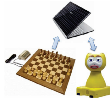
Fig. 1. System setup: a laptop, an electronic chessboard and the iCat robot.
