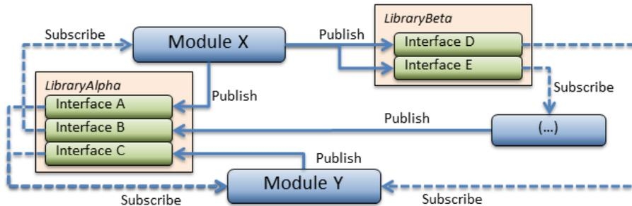
Fig. 2: Example scheme of how different modules publish and subscribe to events.
