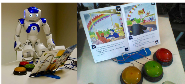
Figure 2: CoReader platform; Left image shows the robot with the book and buttons; Right image shows the view from the robot's bottom camera looking at the book accompanied with ARTags
