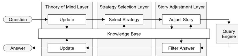
Figure 1: Deceptive Virtual Agent's two pass control layered architecture
