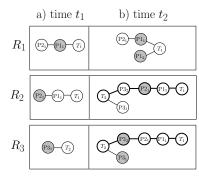
(b) Network graphs for the 3 robots shown in Fig. 2a. The shaded vertices indicate positions that the robots can convert into coordinates. Edges between vertices indicate connectivity. The solution found is outlined in bold.
