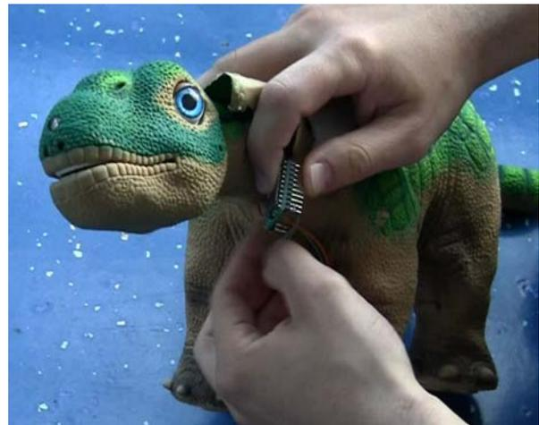
Figure 2. Integration of a Bluetooth module inside Pleo's body.
