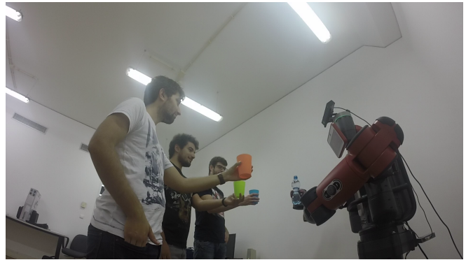
Fig. 1: Scenario layout. The robot on the right serves each of the users on the left. The cups are filled by no particular order and the participants should respond to the robot's movement.
